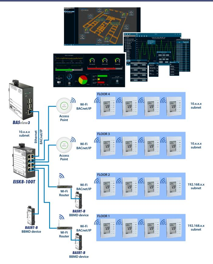
NOTE: Using a Wi-Fi router creates an additional subnet between the wireless network and the wired Ethernet. As is usual for any BACnet communication over subnets, BBMD devices are required on each subnet. BBMDs are not required if a Wi-Fi Access Point, that extends the same subnet as the wired Ethernet, is used to integrate the wireless thermostats.
