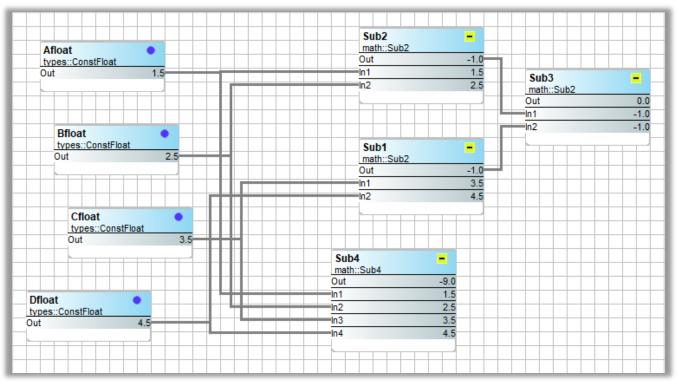
The subtract (Sub) components are also easy to work with but notice that cascading components do not yield the same results. The first input (In1) is the minuend, and all other inputs (In2, In3, In4) are subtrahends leading to outputs which represent the difference.
