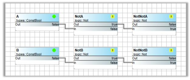
There are two Boolean variables A and B which are set to be false. Both feed a Not component that is usually called an inverter because it changes the initial variable to the opposite state, which it true. Going into another inverter changes the state back to the original states of A and B.
