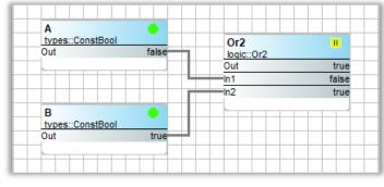
For an OR gate, If A is false and B is true, then the output is true.
