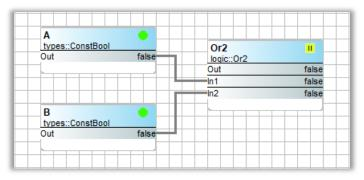
The OR component if frequently called an OR gate. If A is false and B is false, then the output is false.
