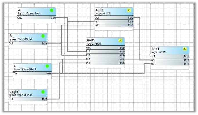
Four-input AND gates exists, but unused inputs must be accommodated by creating a Logic1 constant that is tied to all unused AND gate inputs, otherwise the AND gate outputs would be permanently disabled.
