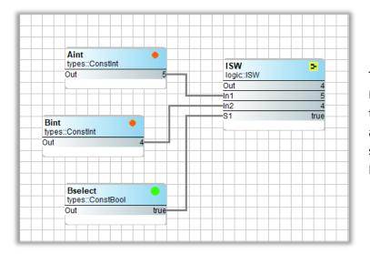
The integer switch (ISW) is much like the BSW and ASW. The selector is a Boolean, but the inputs are integers. The output remains an integer. The logic is the same. If the selector (S1) is true, then the output follows In2, otherwise it follows In1.
