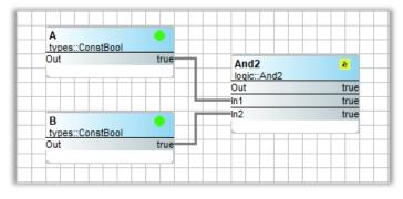
For an AND gate, If A is true and B is true, then the output is true.
