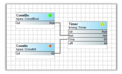
The timer component will count down from a predetermined amount when the Run input is true. A constant integer component was used to set the time, although the Timer component can be internally configured. The output will remain true during timing and transition false upon completion or if the Run input goes false. To begin a new timing period, the Run input must be cycled.
