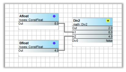
Division is also straight forward. Input 1 (In1) is the dividend, input 2 (In2) is the divisor, and the output (Out) is the quotient. Dividing by zero will result in the pin Div0 being set to true.
