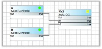
For an OR gate, If A is true and B is true, then the output is true.
