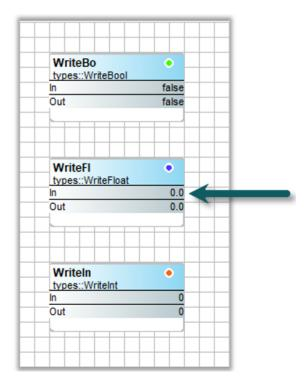
In a similar manner, there are write components for each variable type. Unlike the constant components, these write components have an input slot. The value of the input will be saved if the application program is saved. Other than the input slot difference, the constant components and the write components function the same.
