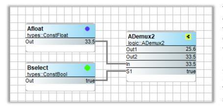
The analog de-multiplexer has only one input (In) one selector (S1), and two outputs. When the S1 is false, Out1 reflects the input. When S1 is true, Out1 will reflect the input just before the selector changed state, and Out2 will reflect the instantaneous value of the input. This component can be treated as a sample-and-hold detector.
