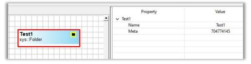
Rename the component in the Properties Pane to "Test1," and press return. Double-click the component, and a new blank wiresheet appears which shows the contents of your new folder. At the top of the wiresheet is a new tab with the name of the "Test1" folder.
