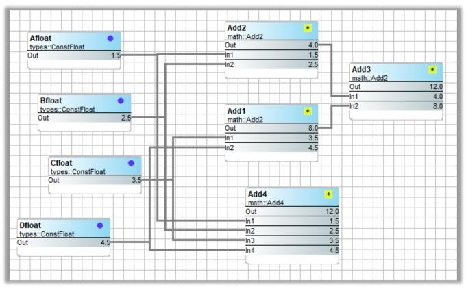
The addition (Add) components are straight forward. You can cascade two-input Add components, or you can use a four-input Add component. All inputs and outputs are floats.
