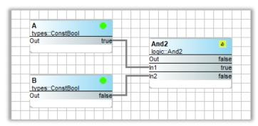
For an AND gate, If A is true and B is false, then the output is false.
