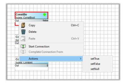
You can set the value of the constant by rightclicking on the component and the selecting Actions. For the ConstBool components, your choices are True, False or Null. Null is seldom used.
