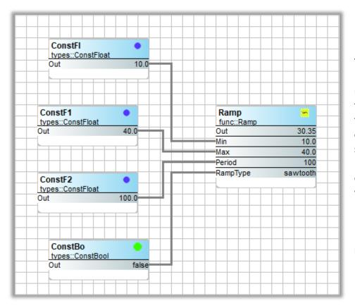
The Ramp is similar to the IRamp, but the Ramp has mostly float settings and a float output. The output of the Ramp can be configured or programmed for either a sawtooth or triangle wave. Increasing the period slows down the speed of the Ramp within the limits of Min and Max. Notice that although the Period is a float, the input to Period will be rounded to the nearest integer.
