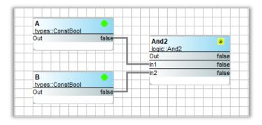
The AND component if frequently called an AND gate. If A is false and B is false, then the output is false.
