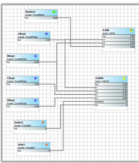
Similar in operation to the binary switch (BSW) is the analog switch (ASW). Instead of Boolean variables, the inputs are floats, but the selector (S1) is a Boolean variable. With S1 set to true, the ASW output selects input 2 (In2), otherwise Input 1 (In1) is selected. Therefore, the ASW selects one of two input float options.
