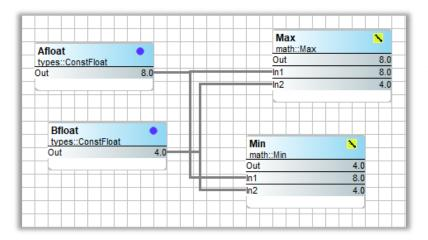
The Max component output (Out) reflects the maximum values of the two input floats (In1, In2), while the Min component reflects the minimum value of the two inputs.
