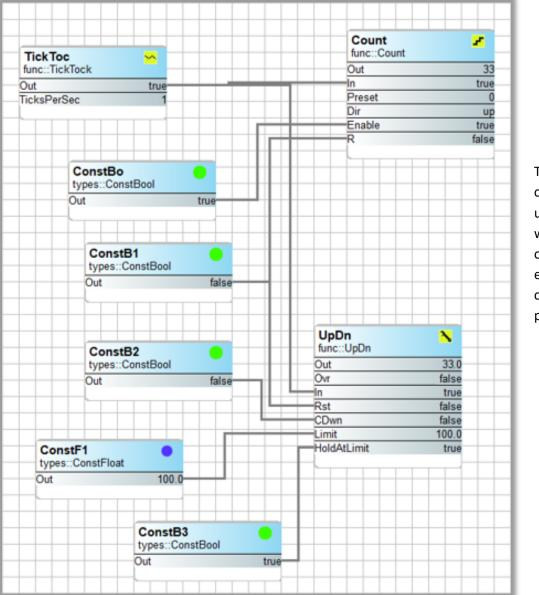
There are two counters. Count is an up/down counter with an integer output. It must be enabled to count. It can be reset to 0 or preset.
