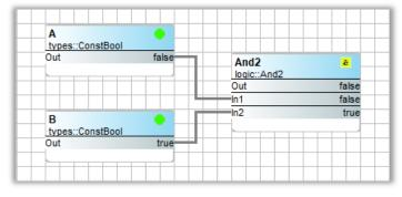
For an AND gate, If A is false and B is true, then the output is false.
