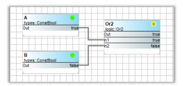
For an OR gate, If A is true and B is false, then the output is true.
