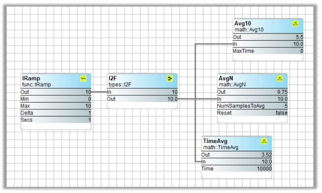
In this example, three averaging components are compared. The Avg10 averages over ten samples, but the data must change to trigger a new sample. The AvgN component can be configured for the number of samples, but it samples every scan and not just on a change in value. The TimeAvg averages over a fixed period of time which is configurable. The output does not change until all samples are obtained.
