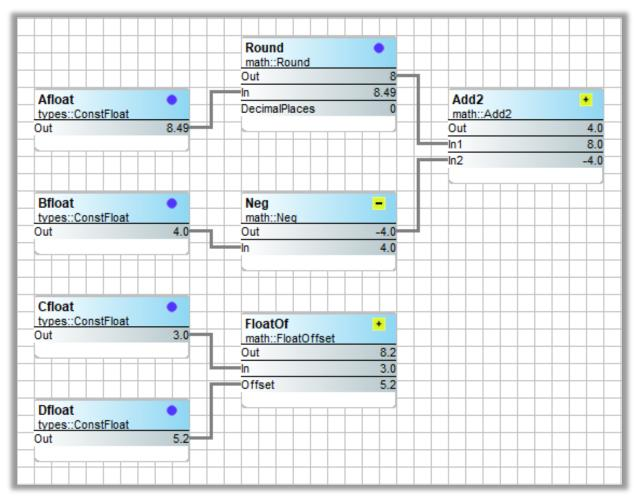
Using the Round component, you can round-off the value of a float to the closest integer value, but the output will remain a float. Using the Neg component, you can append a minus sign to a float with the output remaining a float.
