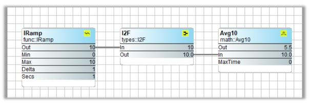
The Avg10 components averages the last ten input values and sends the result to the output. To demonstrate this, an IRamp is configured to create a triangle wave with a minimum value of 0 and a maximum value of 10. Increments are set to 1. When the IRamp reaches 10, the Avg10 component would have averaged 10, 9, 8, 7, 6, 5, 4, 3, 2, 1 for a value of 5, which appears in the output.
