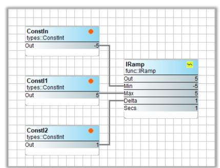
The IRamp provides a triangular output ranging from Min to Max with increments of Delta. These paraments can be configured or programmed as shown. The time increment must be configured having the units of seconds. Notice that all the configurable settings are integers, as is the output.
