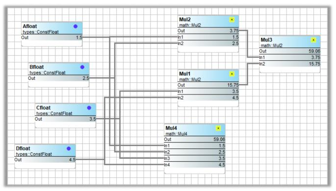
Similar to addition, float variables can be multiplied either by cascading multiply (Mul) components or by using a single larger multiplier component. All inputs and outputs are floats.
