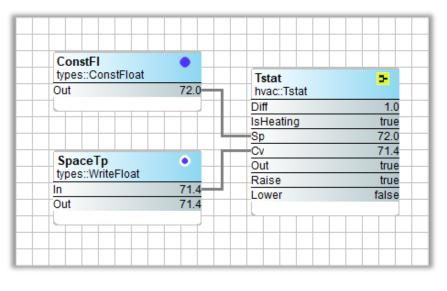
The Tstat is an on/off temperature controller for either heating or cooling. For heating configure, the IsHeating is set to true. The deadband can be set by the Diff value. If the controlled variable (Cv) deviates from the setpoint (Sp) by half the Diff value, the output (Out) will become true and stay set until Cv deviates from the setpoint by a like amount in the other direction. In this way, Diff also provide hysteresis. The Raise and Lower outputs are a function of the IsHeating setting.
