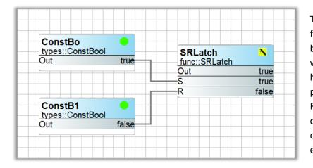
The SRLatch appears to be a straightforward logic block. The output would become true if the set (S) pin is high and would go low if the reset (R) pin goes high. However, both the S and R pins are positive leading-edge sensitive. Regardless of their steady-state condition, the output (Out) will only change on the false-to-true transition of either input.
