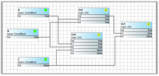
Four-input OR gates operate the same allowing more variables to be added to the logic. With OR gates, unused inputs can be left unconnected because unused inputs default to false.
