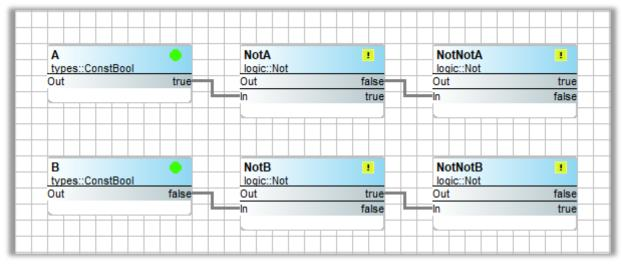
Variable A is now set to be true. Notice in the second panel the output of the first inverter changes the value of A to a false, while the second inverter restores the state of A back to true.
