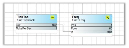
The TickToc component provides a convenient clock from 1 to 10 pulses per second. However, because the controller scan time and other processing overhead, it is recommended to use its default value of 1 second. More accurate timing is available from a real-time clock.
