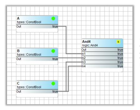
Here is another way of handling an unused input when three variables are connected to a four-input AND gate. Attach the unused input to one of the variables. It does not matter which one is used.
