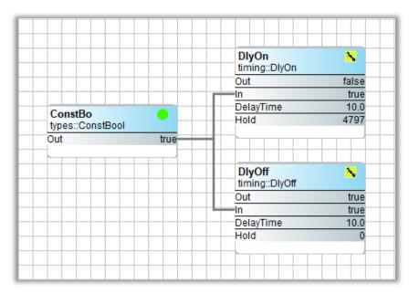
The DlyOn component is an on-delay timer which begins timing on the false to true transition of the input. Once the time (as shown is the Hold slot) goes to 0, the output will become true. This delay time is configurable. In this example, the delay timer is still timing after the input when true 4.8 seconds ago.
