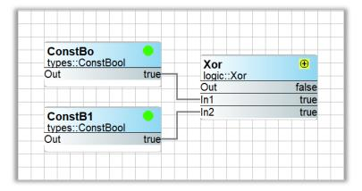
An Exclusive OR is very similar to an OR except for the condition when both inputs are true. In this case, the output is false. An XOR solves the problem of A or B, but not both.
