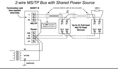
For MS/TP devices that use a power source separate from the BASRT-B
