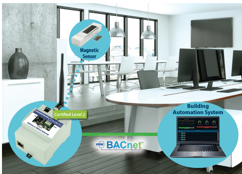
The window monitoring solution integrates an EnOcean solar-powered window sensor with an EnOcean to BACnet gateway, allowing a building automation supervisor to manage a window's open/close status in real time.
