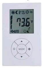
The BAScontrol-E36 supports a wall setter option. This four-wire powered serial port connection can accommodate one Contemporary Controls' BASWS-M wall setter. The wall setter has a large LCD display with programmable numeric characters and icons to show mode of operation, setpoint, and measured
