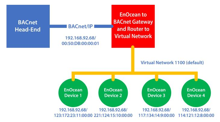
The BACnet head-end sees the EnOcean devices as standard BACnet devices through the EnOcean to BACnet Gateway, which acts as a BACnet router to the virtual network containing the EnOcean devices. Each EnOcean device has the IP address of the gateway and appears to be on network 1100 with an automatic BACnet MAC address.
