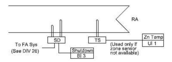
For return air, you have a provision for a return air temperature sensor (TS) that can be in the return air duct or you can use a space temperature sensor that is mounted in the wall setter. A shutdown provision such as a smoke detector (SD) is provided to meet local fire code requirements.
