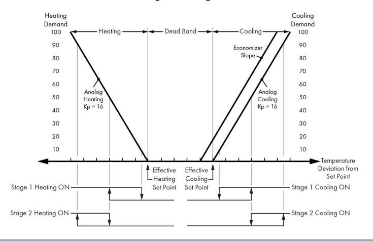
Economizers add an early stage of free-cooling assuming the outside temperature (dry-bulb) or outside humidity (dry-bulb and relative humidity) are conducive to free-cooling. An additional PID component and other logic are used for economizing.
