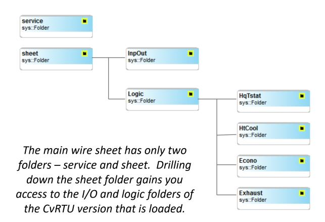
InpOut – All real, virtual and web components are located in one folder
