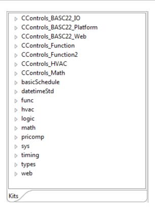
The Kits pane shows you all the kits installed on the controller. Expanding a kit gains you access to the components within the kit.
