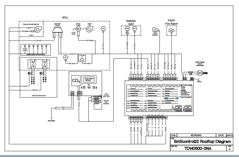
To assist the panel builder in designing a panel, a sample wiring diagram is provided in .dxf format showing the interconnections between the controller and recommended ancillary equipment.
