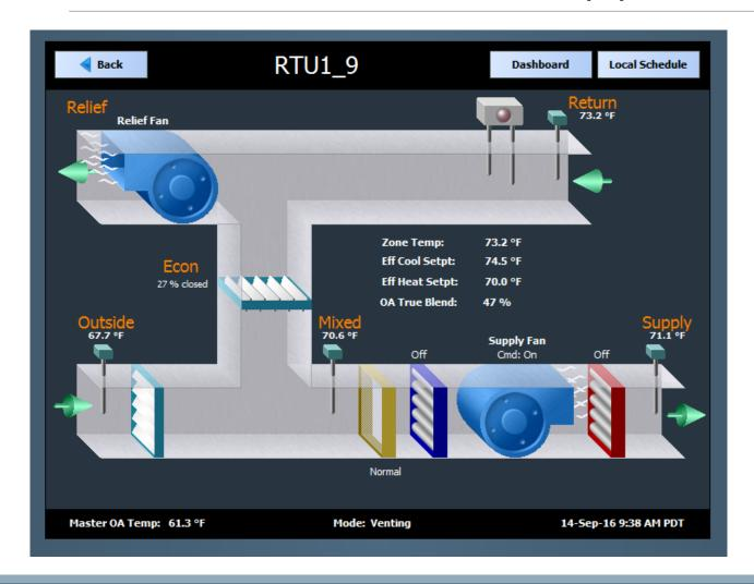
The CvRTU series provides five pre-built control applications for rooftop units (RTUs) that will execute on a Contemporary Controls' BAScontrol22 BACnet/IP Sedona controller. Pre-built applications speed up installation time by only requiring configuration during installation.
