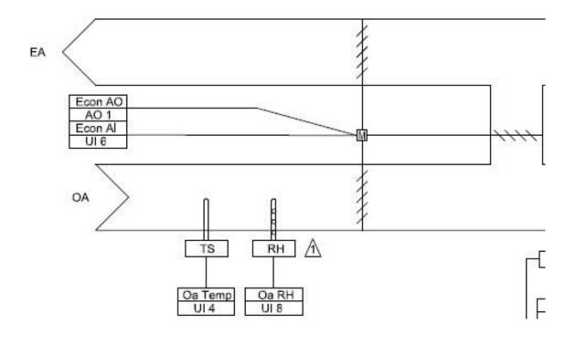
You can also have a dry-bulb economizer requiring an outside air temperature sensor (TS), an enthalpy economizer requiring a relative humidity sensor (RH) in addition to the dry-bulb sensor or no economizer at all. A proportional damper actuator must be provided which has analog position feedback.
