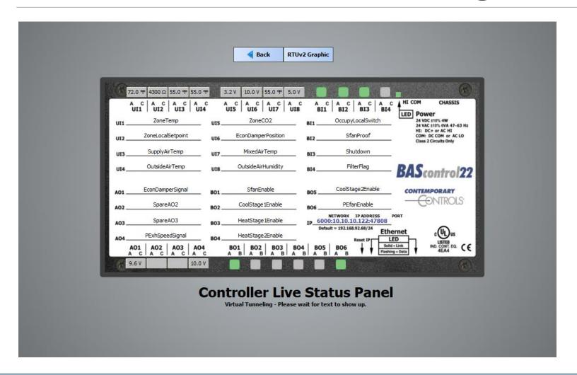
Each controller in a system can have its own dashboard showing live status of its real points both analog and digital.
