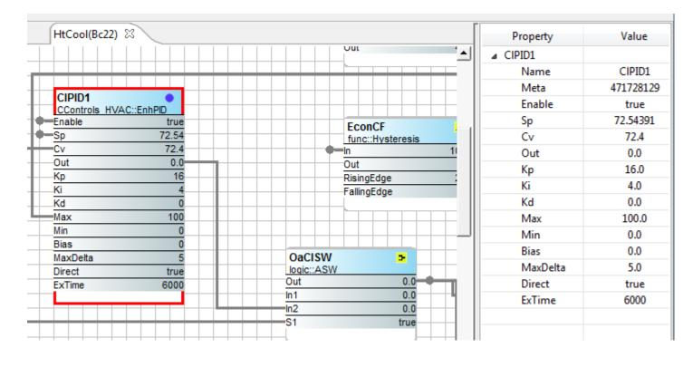
By highlighting a component, its properties can be viewed in the Properties pane. This is where PID settings or any other property can be changed. Any changes are temporary until the application is saved to the controller.
