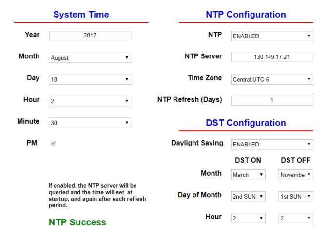
System time can be set manually or automatically when there is Internet access to a network time protocol (NTP) server. The time zone must be set and daylight saving time (DST) dates must be entered. In the event of a power loss, system time is maintained for up to seven days.
