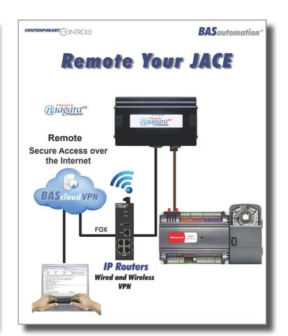
Our EIPR-V wireless router provides a secure VPN connection to the JACE in conjunction with our BAScloudVPN cloud service.
