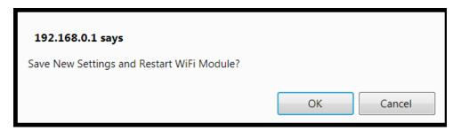
When *OK* is clicked, a confirmation is displayed to indicate configuration is stored in the thermostat's internal memory. After reboot, the new thermostat credentials will be *admin* for username and the newly configured Access Point's password for password.
