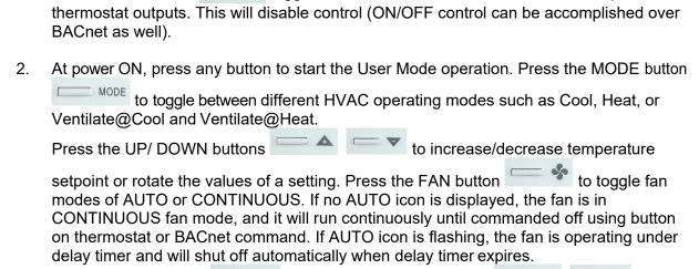
The POWER button toggles between ON or OFF states to start / stop the
