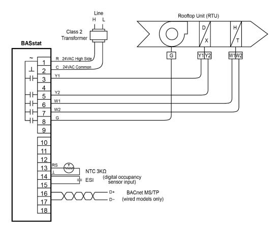
Wiring: 14 to 22 AWG wires or 1.5mm2 wires
